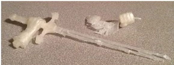
These are parts that were printed far too thin for the printer to be able to handle.
