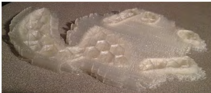
The Result of a major jam halting the printer. That is 15 wasted hours right there.
