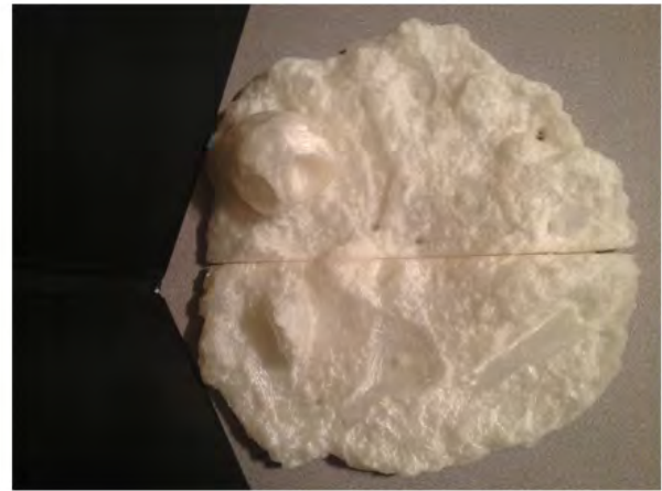
Here you can see how large objects shrank and warped while being printed, the two halves no longer line up despite being razor straight.
