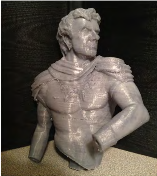
Another example of minor jams during printing that result in a surface full of gaps and errors.
